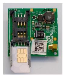
Normally the RTU will be supplied with a SIM Card fitted and ready for operation for the area of the world for which it was ordered.
