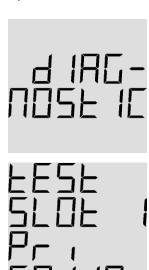
'To enter "Diagnostic Mode" press and hold both the "Fill" and the "Mode" buttons simultaneously until the "Diag-nostic" prompt appears on the display.
