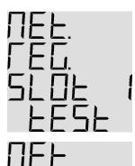
The "Network Registration" screen is displayed while the DPW900 series device attempts to register with the communications network.
