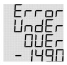
Channel 1 shows "Error" as it is measuring a signal of 25mA. Channel 2 shows "Under" as it is measuring a signal of 0mA. Channel 3 shows "Error" as it is measuring a signal of 25mA. Channel 4 shows "-149.9" as it is measuring a signal of 0mA (-149.9 inches is ¼ of the spanned 0-600 inches measurement range below 4mA, hence the negative displayed value).
